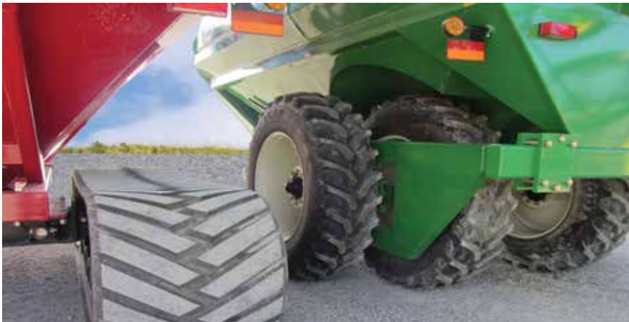
Today's large grain buggies must have tracks or walking beam axles with large tires to minimize soil compaction which is especially important as we move to minimum or no-till practices.
