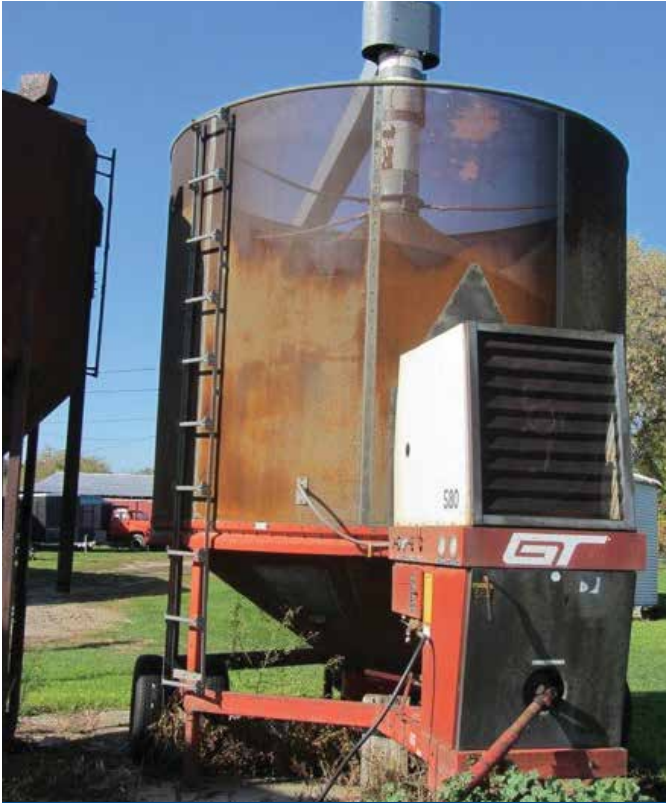
This older batch-type dryer that is PTO-powered by a tractor is still in use.
