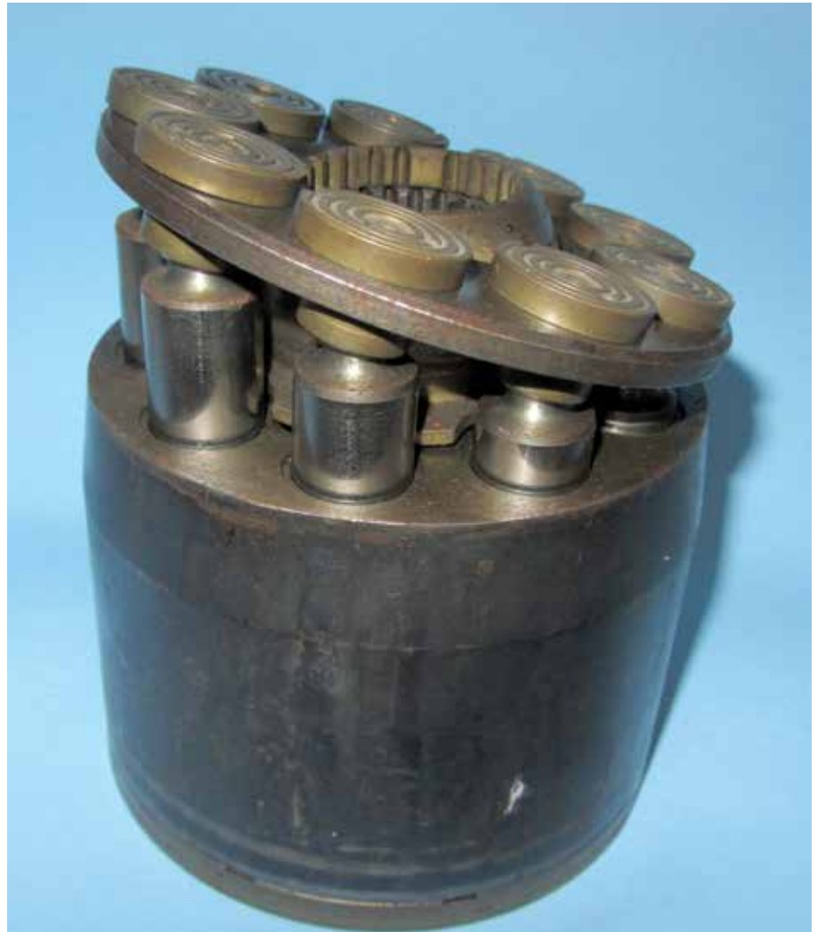
These are the inner workings of a typical, continuously variable output hydraulic pump. Leakage/lubrication is dependent entirely on piston clearance.
