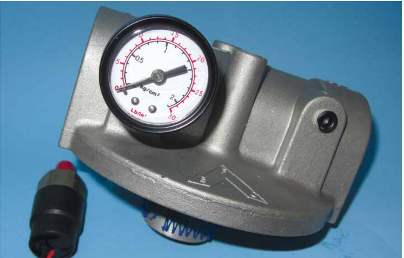
A pressure gauge will indicate fluid bypass and/or filter condition. A prewired red light from a pressure transducer is even better.
