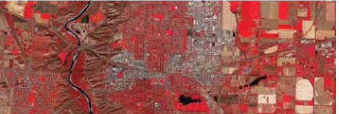
With near-infrared images, dense green vegetation reflects the infrared light, shown on the image as red. This image shows Lethbridge, Alberta in 2015.
