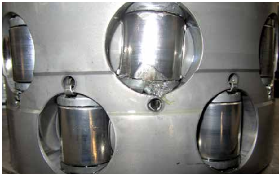
This type of carrier bearing failure causes significant fluid contamination.
